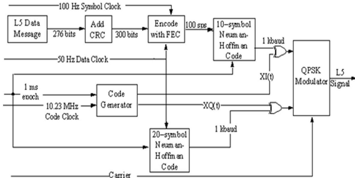
Figure 3-3. Modulation of Signals
