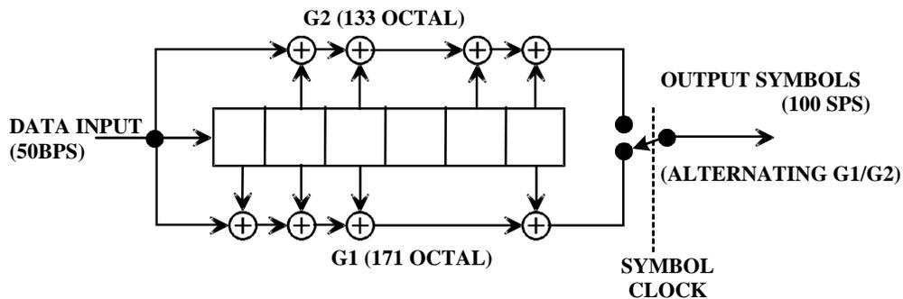
Figure 3-7. Convolution Encoder
