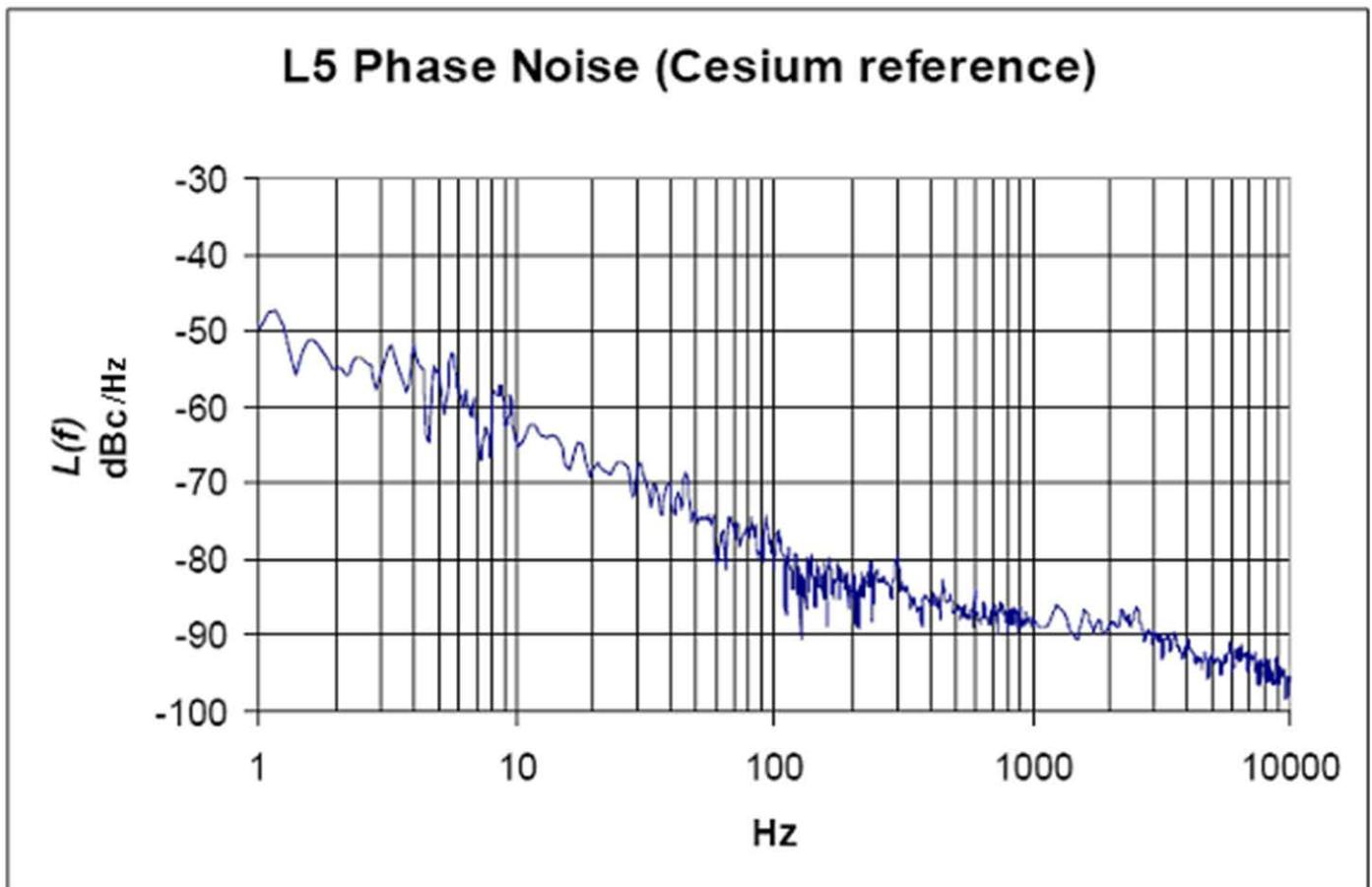
Figure 6-1. Carrier Phase Noise Spectral Density
