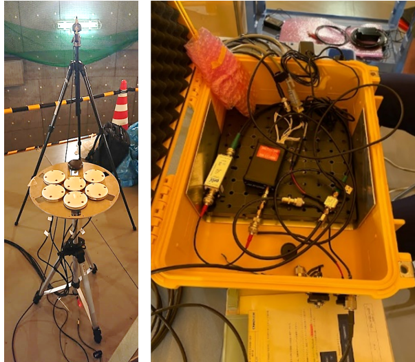
Fig. 5: Equipments and experimental environment (Left: spoofer and antenna array, Right: simulator)
